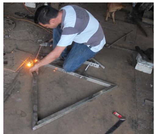
Figure 3. Welding the frame
