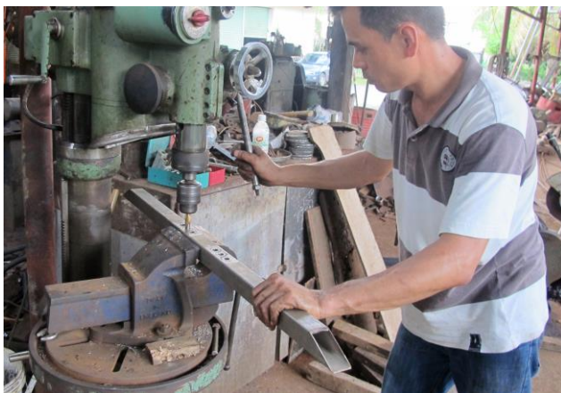
Figure 2. Drilling holes for the clamp
