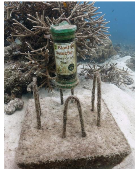
Figure 19. Bomb detector in place
