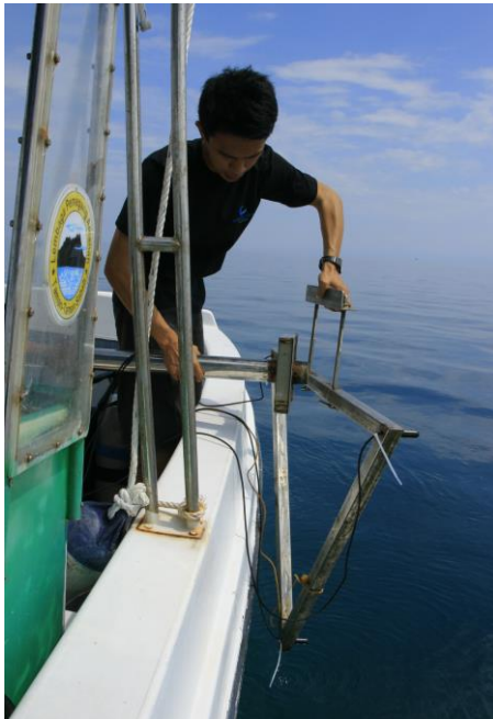
Figure 7. Hydrophone frame being clamped onto a horizontal plate welded onto the bottom end of the pole (left) and ready to be lowered into the water (below).
